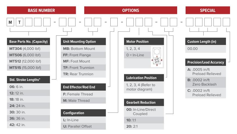
\* MT304 is available with stroke lengths up to 30 in. MT506 and MT512 are available with stroke lengths up to 42 in. MT515 is available with stroke lengths up to 36 in.
